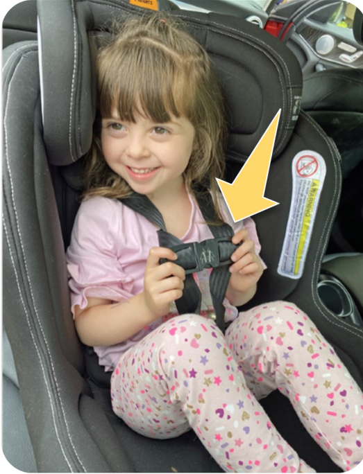
The harness webbing is twisted and is too loose.
