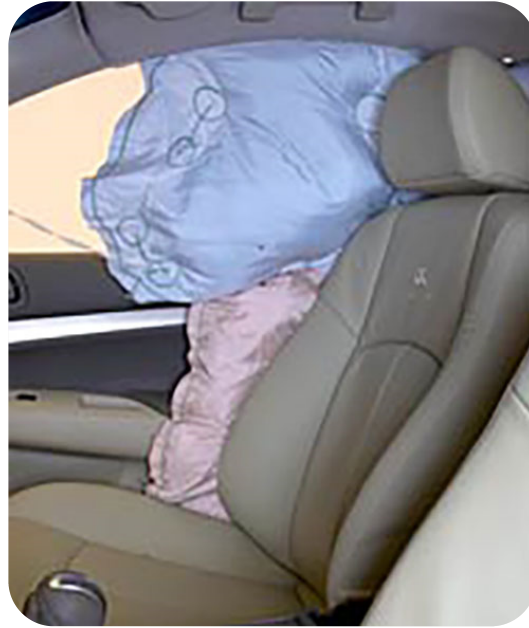
Side air bag that protects the head and chest 2
