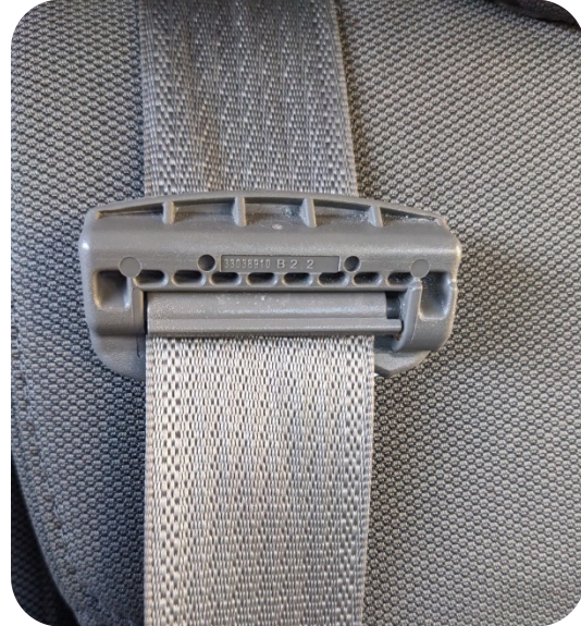
Locking latch plate, front and back views
