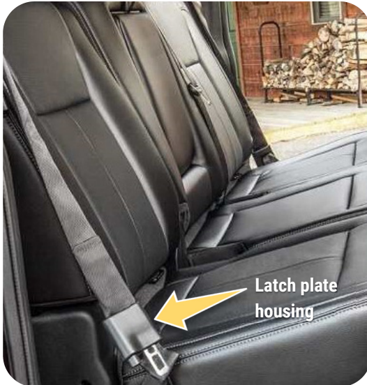
Inflatable shoulder belt showing thicker webbing and large latch plate housing
