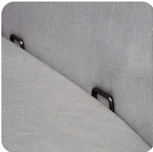
Lower anchors on a school bus seat
