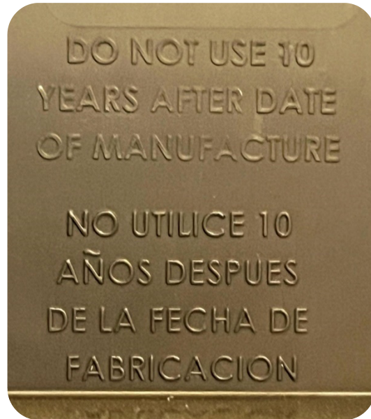
Expiration information stamped into car seat shell
