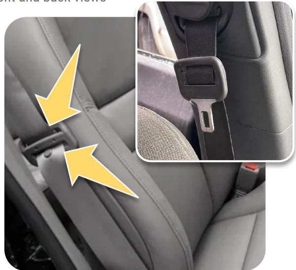
Sliding latch plate with two slots, front and back views
