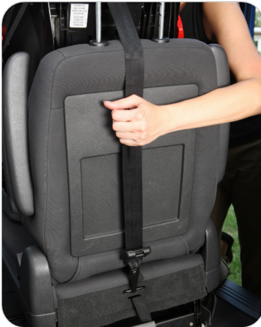
Routing of straight tether under vehicle head restraint
