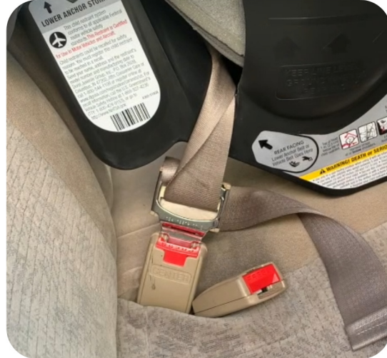
Locking latch plate after flipping
