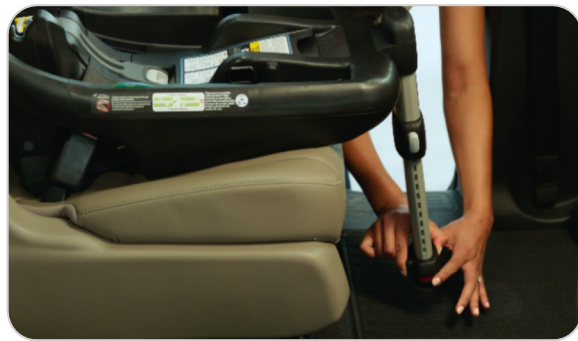
Load leg on detachable base being adjusted to contact the vehicle floor
