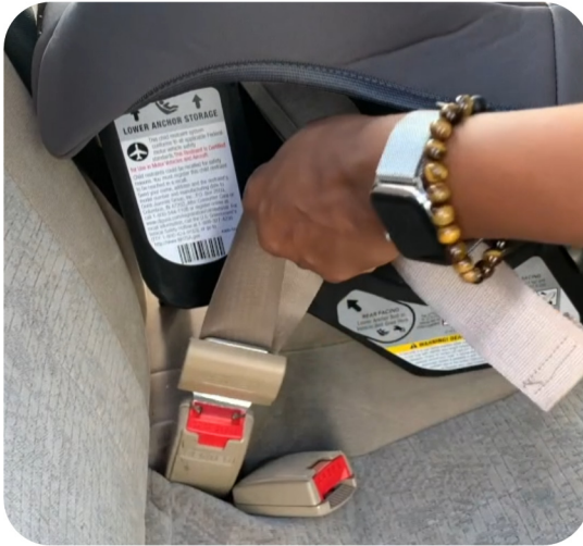
Locking latch plate in normal position
