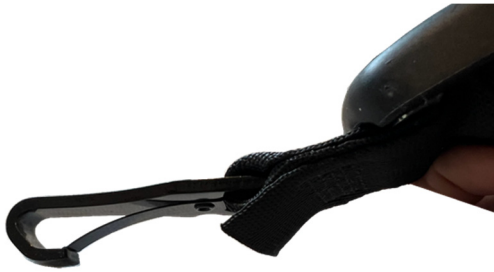
Flexible lower anchor attachment system with hook style connectors
