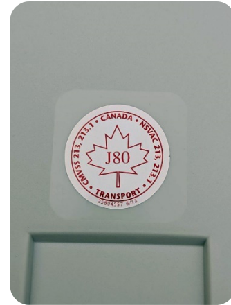
Canada's National Safety Mark required for all car seats and booster seats
