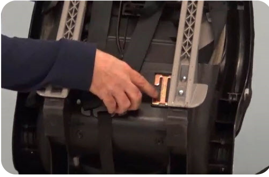
Locking clip, stowed on car seat
