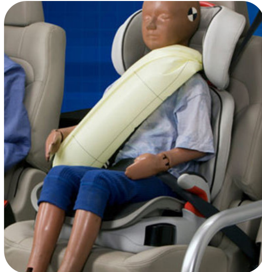
Inflatable shoulder belt, inflated
