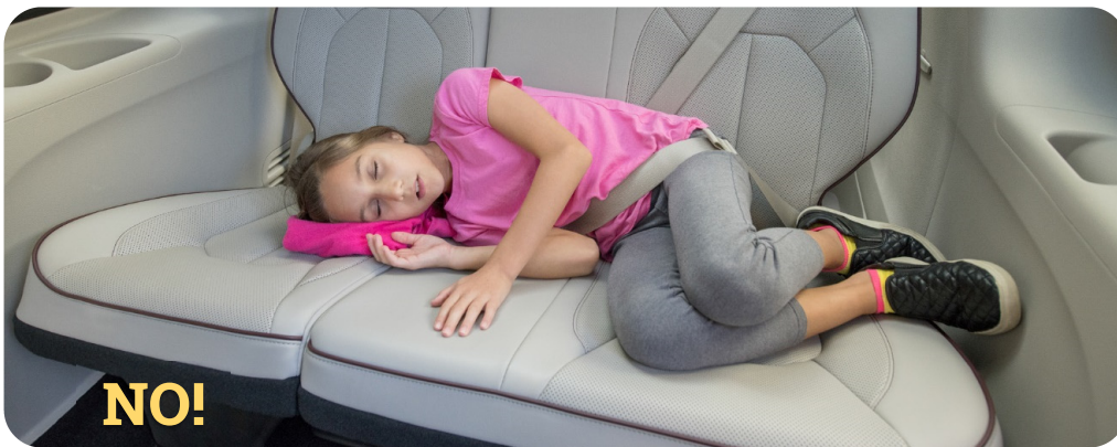
The child is not sitting upright on the vehicle seat. The lap-and-shoulder belt is not correctly used.
