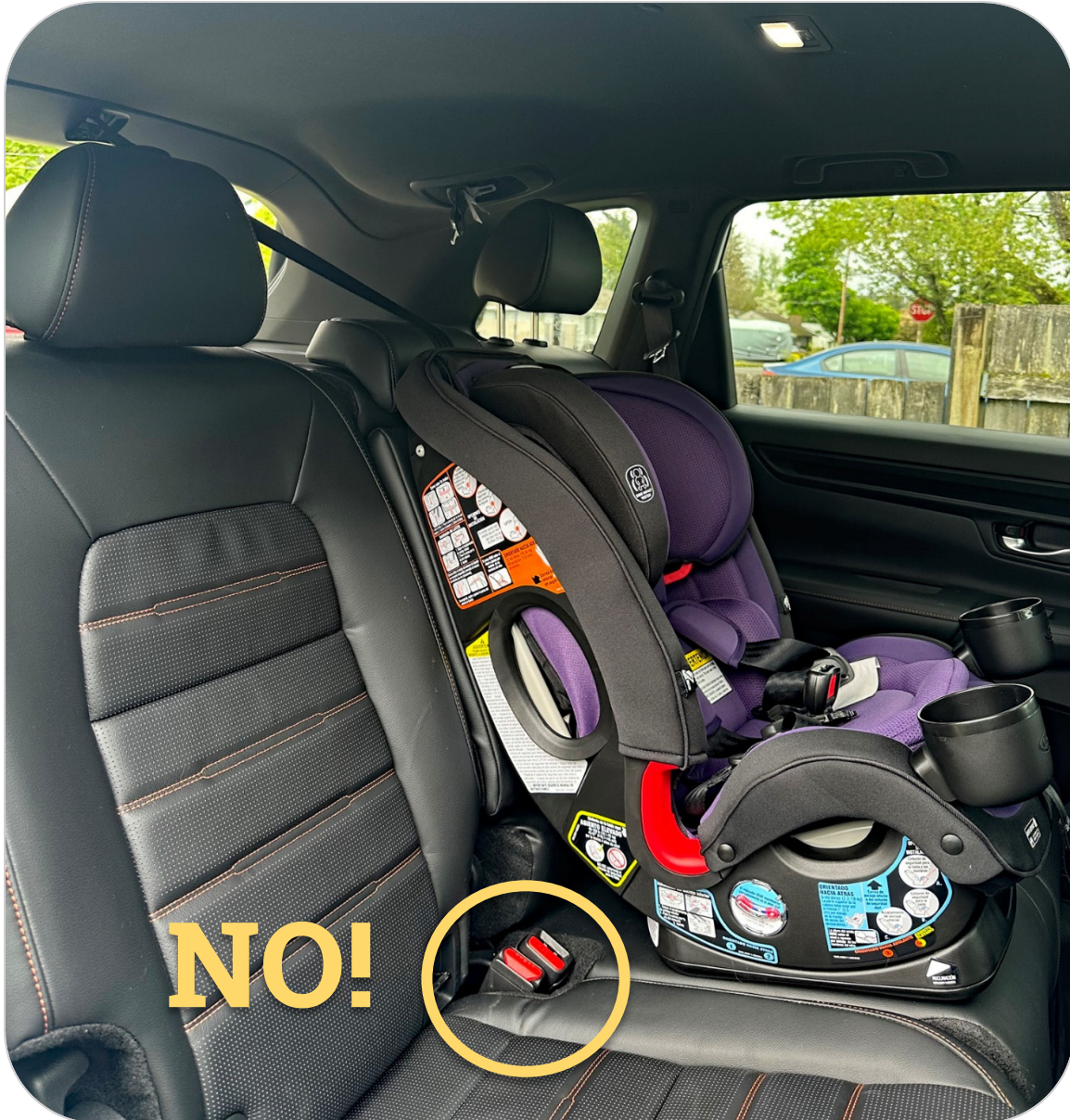
Forward-facing car seat incorrectly secured using only a tether
