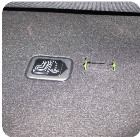
Tether anchor under carpet slit with marking
