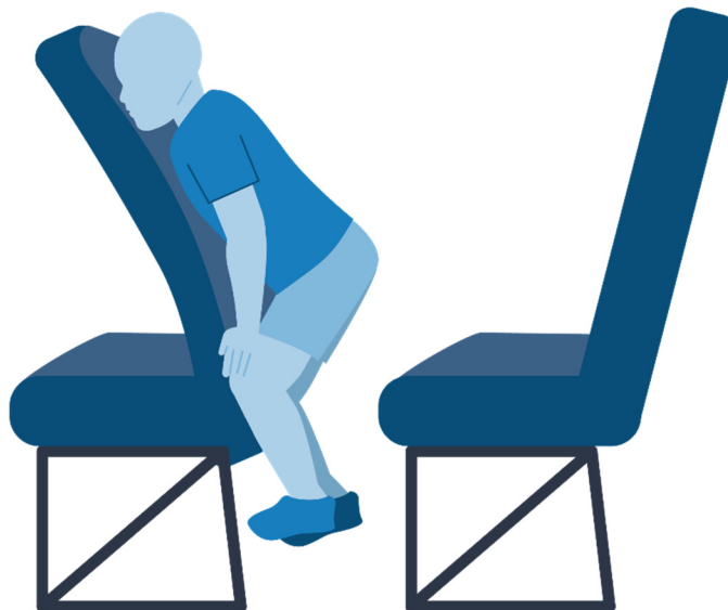
Compartmentalization during a frontal crash
