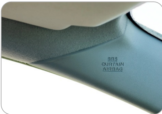
Side curtain air bag marking
