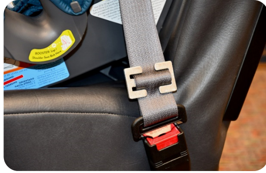
Locking clip in use on lap-and-shoulder belt
