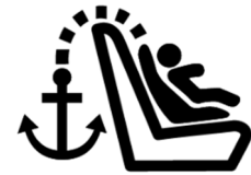
A common marking for tether anchors
