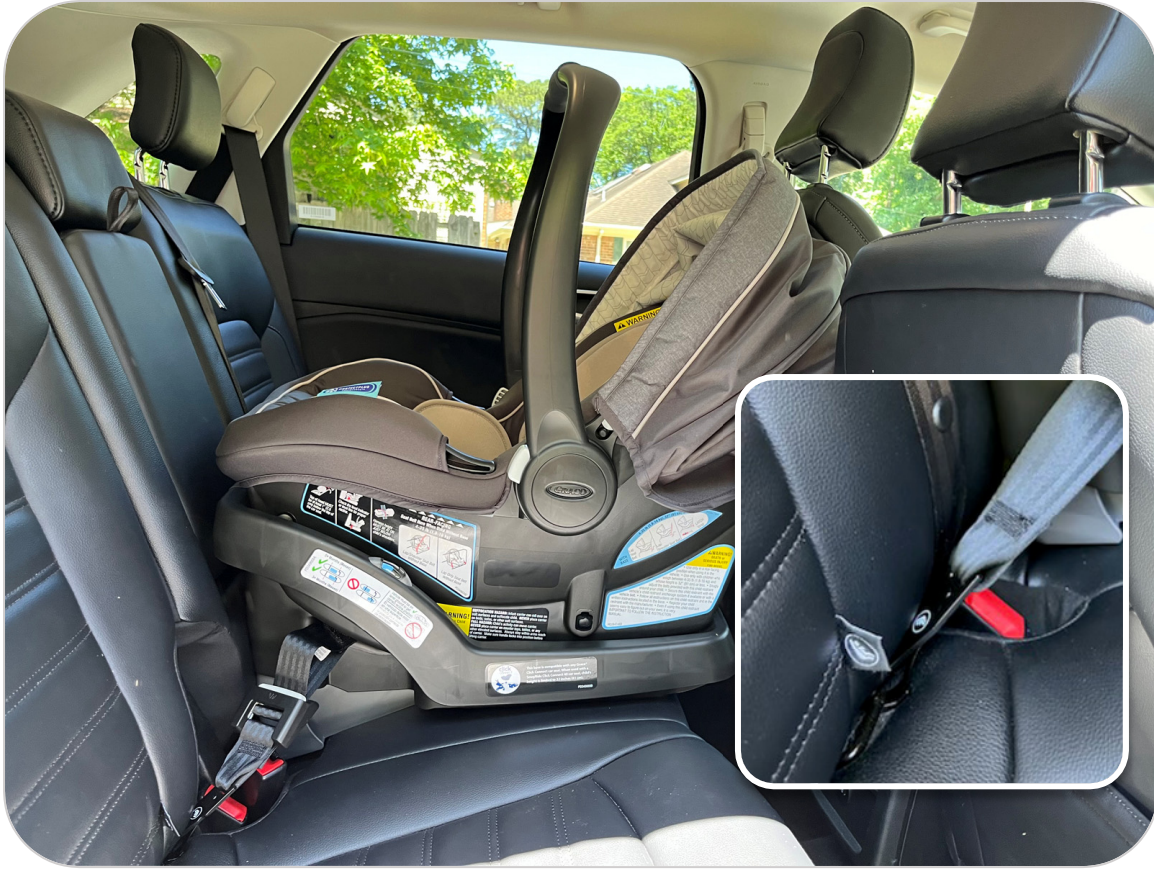
Rear-facing car seat installed in a rear center seating position, borrowing the lower anchors from the outboard seating positions
