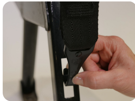
Tether anchor on a school bus seat
