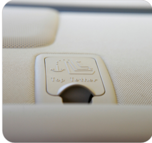
A marking with a symbol and words on a tether anchor's cover flap
