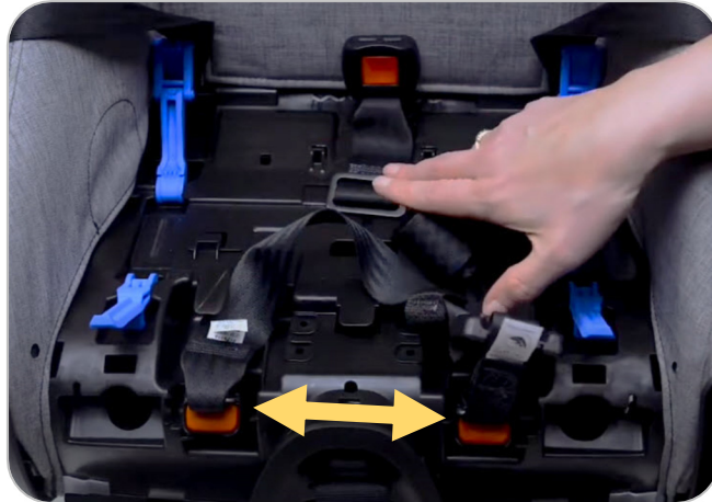
Store unused lower anchor connectors.
