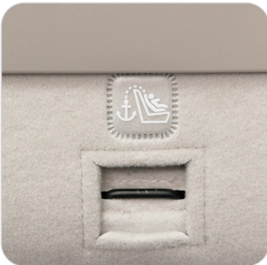
Tether anchor marking above tether anchor
