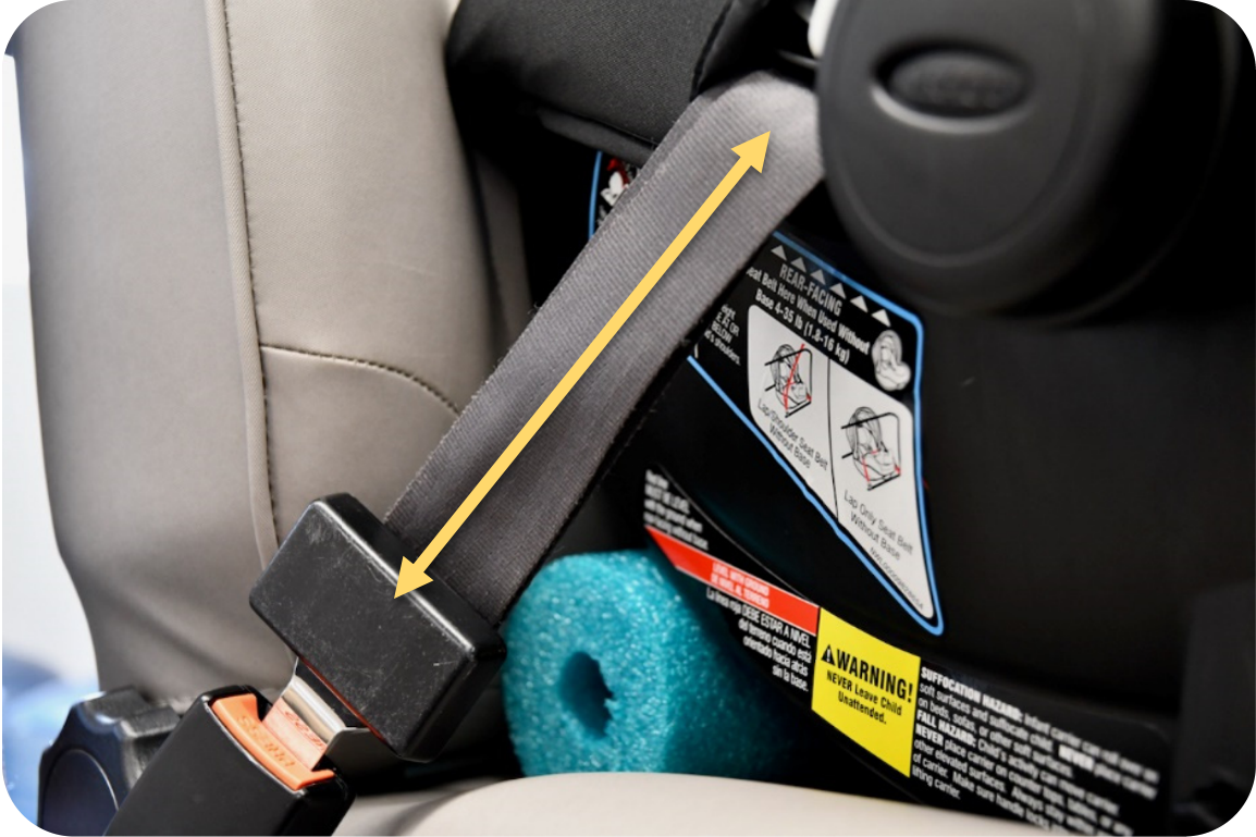
Webbing is parallel with the locking latch plate.
