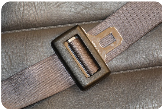
Locking latch plate, front and back views
