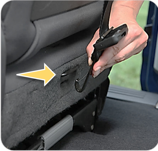
An unmarked tether anchor on the bottom of a vehicle seat
