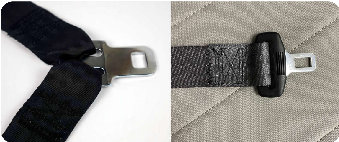
Sewn-on latch plate on lap-and-shoulder belt (left) and on lap belt (right).
