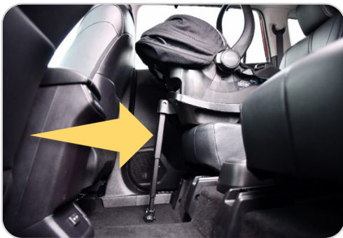
Load leg on detachable base
