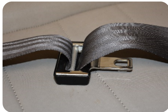
Locking latch plate, front and back views
