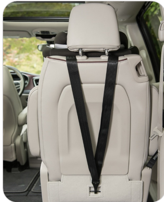
Routing of a V-shaped tether around vehicle head restraint
