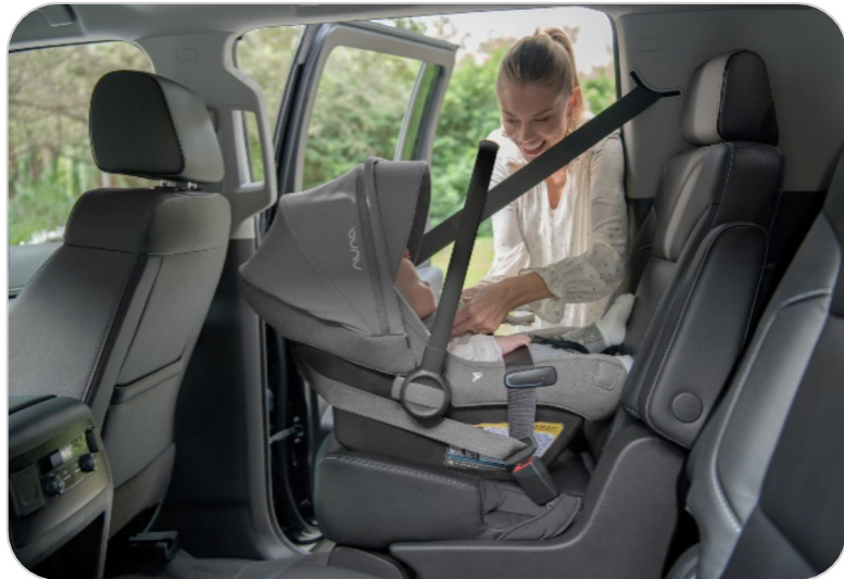
Infant car seat carrier installed without the detachable base using European belt routing
