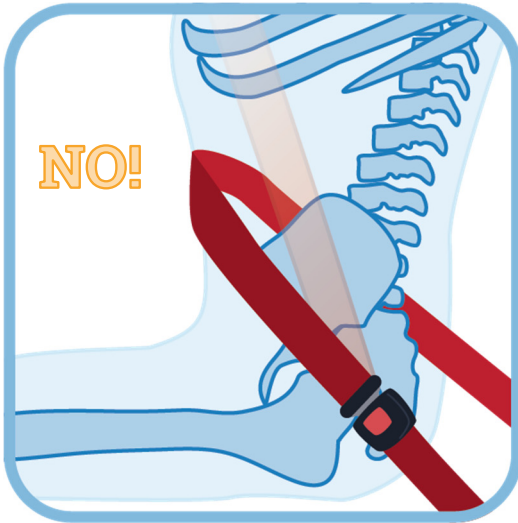
Incorrect placement of lap belt on child slouching on vehicle seat
