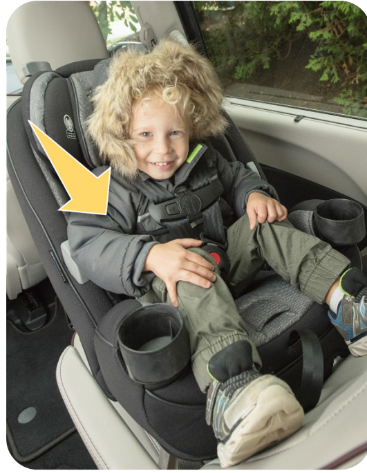
The child is wearing a bulky coat underneath the harness.
