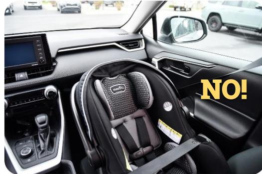
A rear-facing car seat is installed in front passenger seat of a vehicle with an active frontal air bag.
