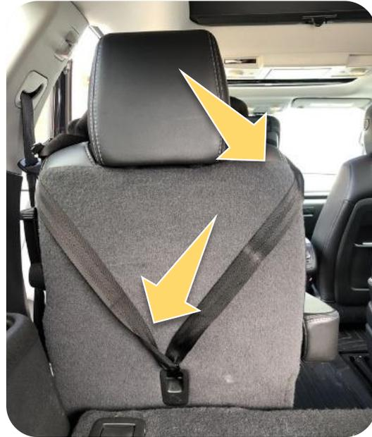
The tether is routed incorrectly around the sides of the vehicle seat, and the tether is twisted.
