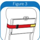
Seats with a recessed tray table – defined as a table that is stored in a cavity with rigid recessed sides. Install the CARES restraint's red loop over the stowed tray table, as shown in Figure 3.
