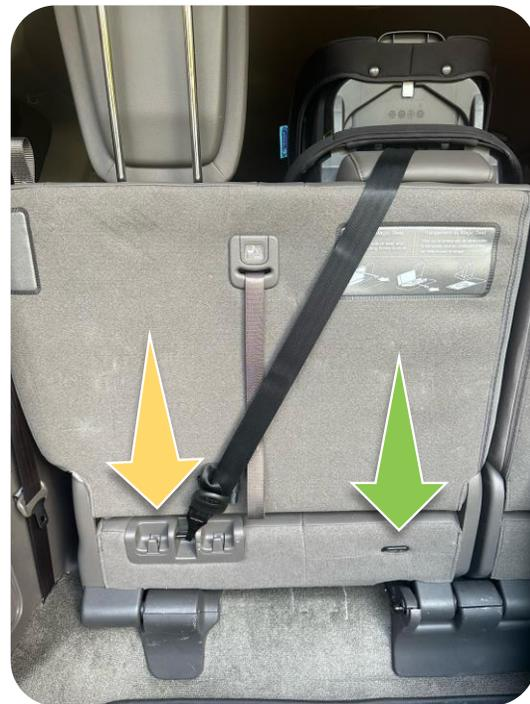
The tether is connected to the incorrect tether anchor. The correct tether anchor is just behind the seating position in this vehicle.
