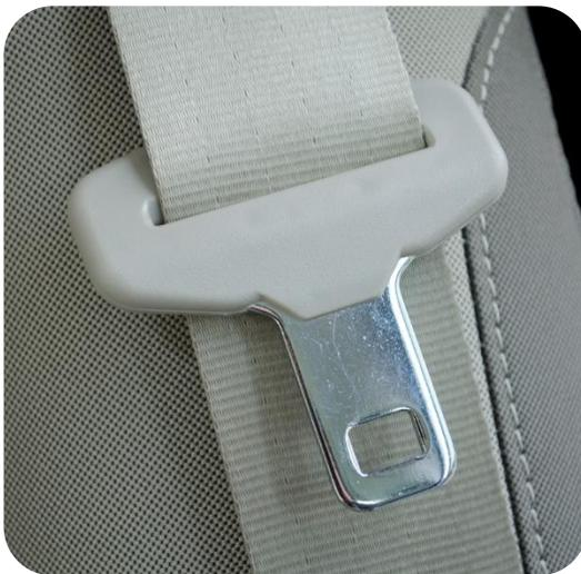
Sliding latch plate with one slot
