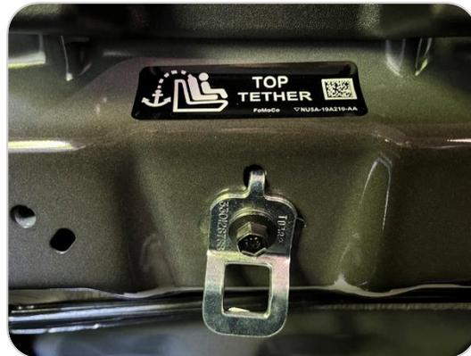
Images from 2024 Ford Maverick vehicle owner's manual (first row) and photos taken inside the vehicle (second row), showing location of tether anchors behind the rear seat.
