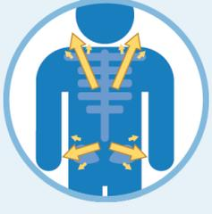
**3** Spread crash forces over a wide area of the body, putting less pressure on any one part.
