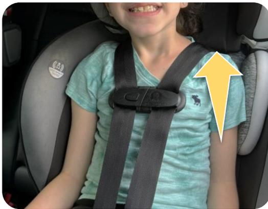
The harness is below the child's shoulders on a forward-facing car seat. The harness should be at or above the shoulders.
