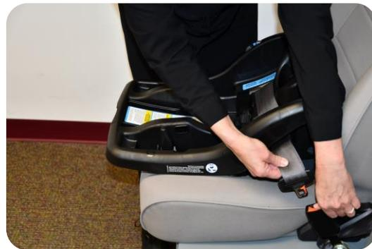
**STEP 4:** Unbuckle the seat belt while continuing to pinch the lap and shoulder belts together.
