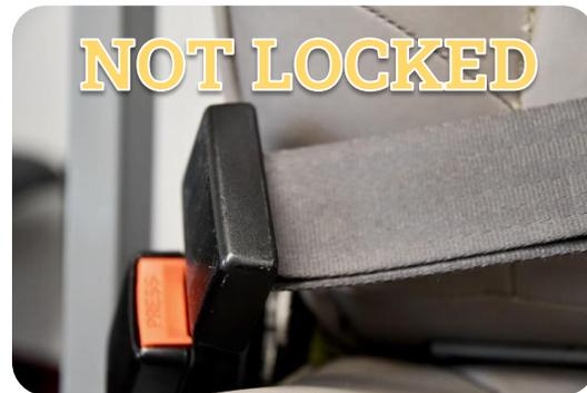
This locking latch plate is not locked because it tilts away from the seat belt webbing.
