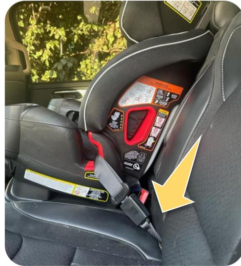
The seat belt is routed through the incorrect belt path (booster seat belt path) for this forward-facing car seat installation. The buckle from the incorrect seating position is being used.
