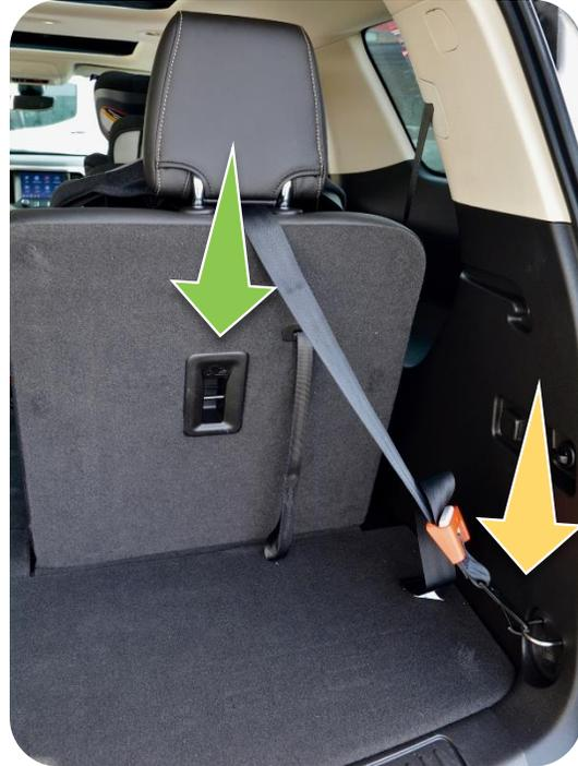
The tether is attached to a cargo hook that is not a tether anchor.
