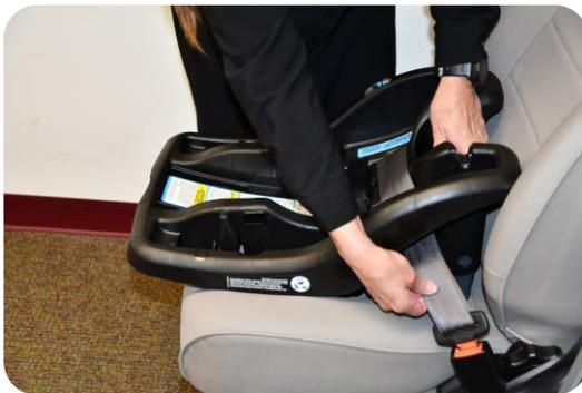
**STEP 3:** Pinch and hold the lap and shoulder belts together near the latch plate.
