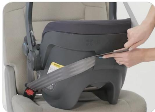
Routing the shoulder belt around the back of carrier
