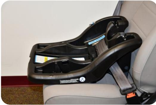
**STEP 1:** Route the seat belt through the correct belt path on the car seat and buckle the seat belt. The seat belt webbing should be flat, not twisted.
