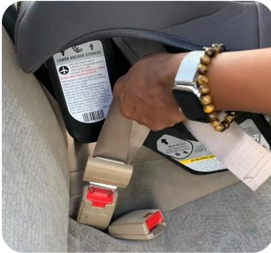
Locking latch plate in normal position
