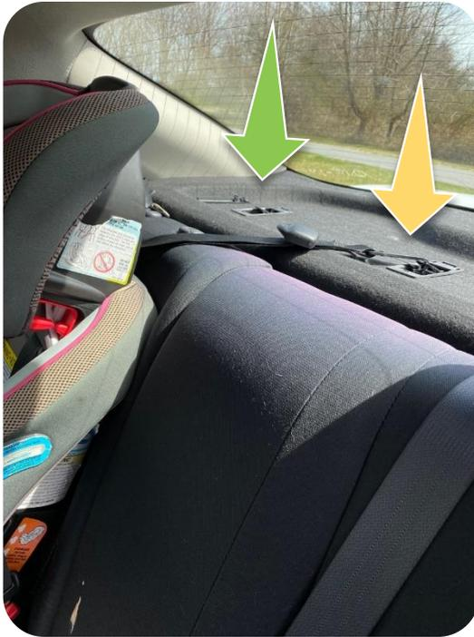
The tether is connected to the wrong tether anchor. The correct tether anchor is just behind the seating position in this vehicle.
