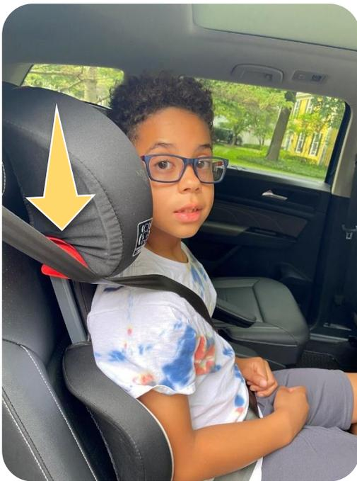
The shoulder belt is not routed correctly through the shoulder belt guide.
