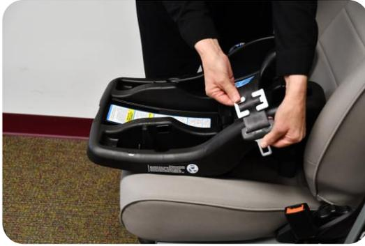
**STEP 5:** Thread the webbing of both the lap belt and shoulder belt through both sets of prongs on the locking clip.
