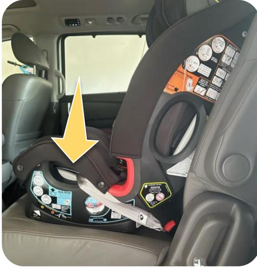
The lower anchor attachment system is routed through the incorrect belt path (rear-facing belt path) for this forward-facing car seat installation.
