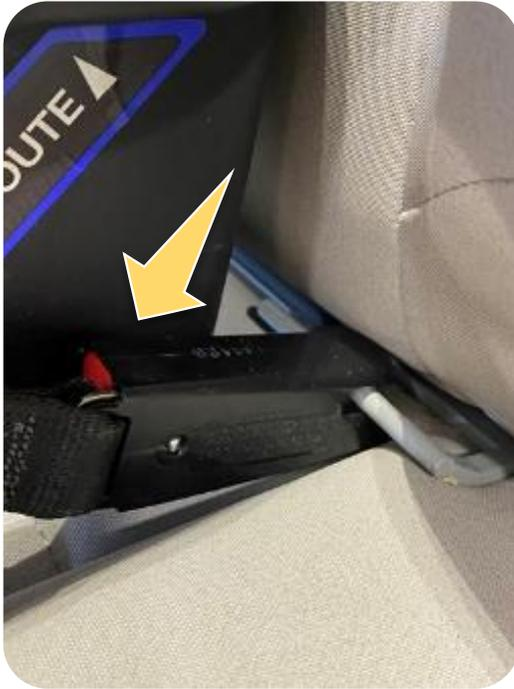
The lower anchor connector is attached upside down.
