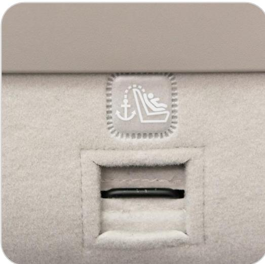
Tether anchor marking above tether anchor
