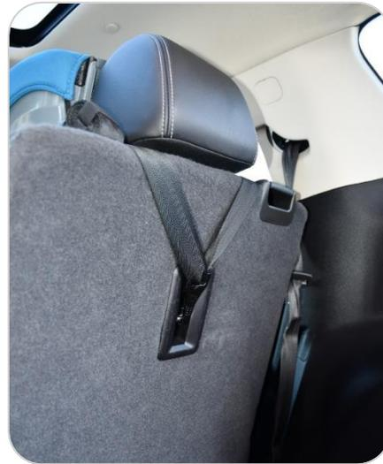
Less often, the webbing is attached to two points on the car seat and the tether hook is free sliding. This type is commonly referred to as a V-shaped tether.
