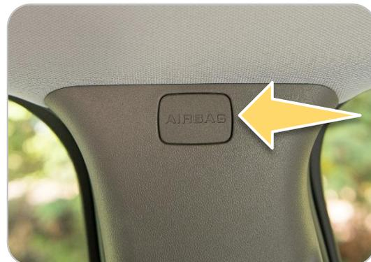
Curtain air bag marking near roofline
