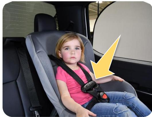
The chest clip is too low. It should be at armpit level. The harness is too high. It should be at or just above the shoulders. The harness is too loose. It should be snug against the child's body.
