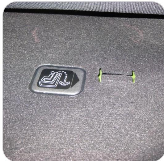
Tether anchor under carpet slit with marking
