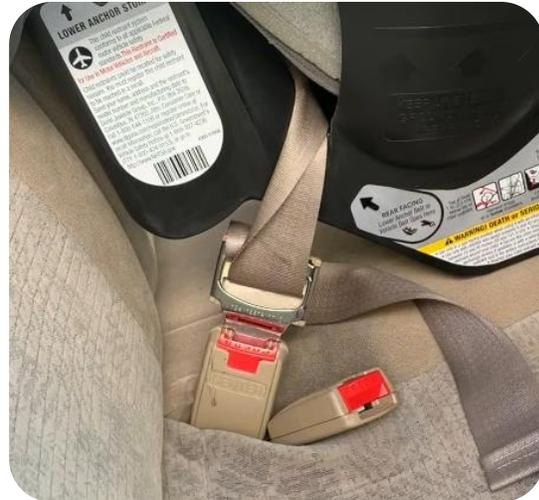
Locking latch plate after flipping
