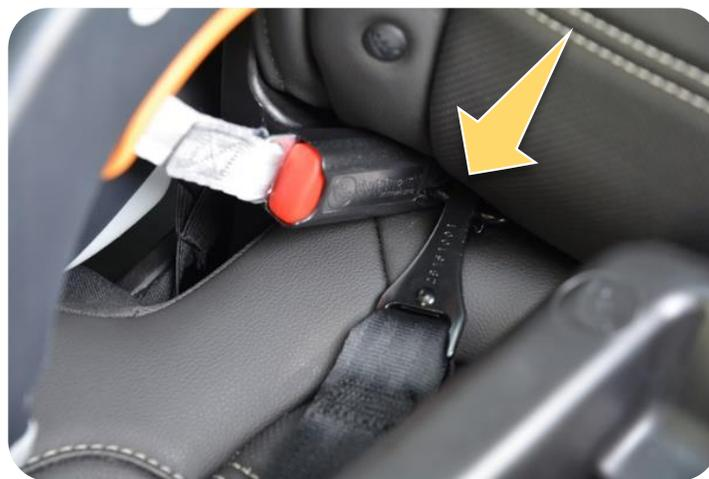
Two lower anchor connectors are attached to one lower anchor.
