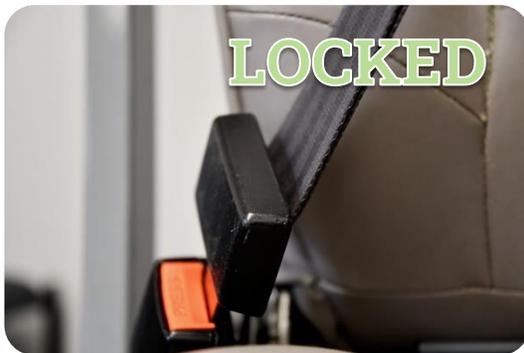
This locking latch plate is locked because it is parallel with the seat belt webbing.
