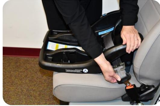
**STEP 6:** Re-route the locked seat belt webbing through the car seat belt path. Press the car seat firmly into the vehicle seat cushion and buckle the seat belt.
