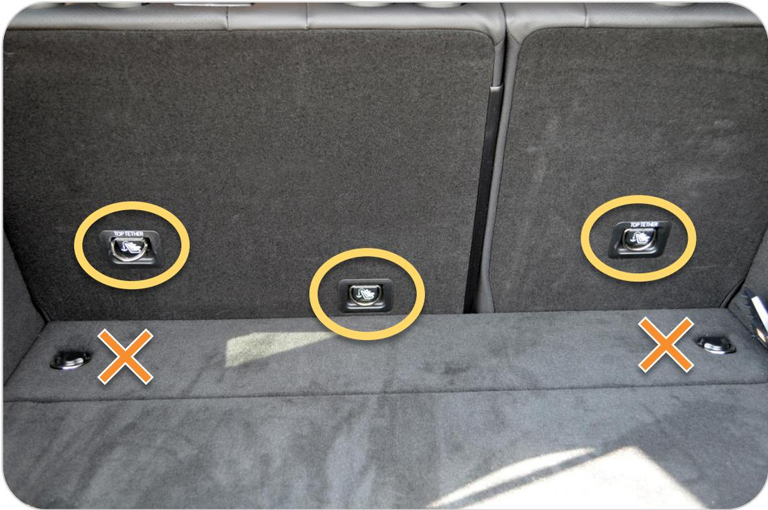
These tether anchors (circled) are on the back of the vehicle seatback. The "X's" mark cargo hooks, which must not be mistaken for tether anchors.
