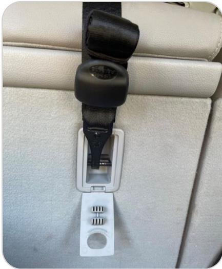
The webbing is usually attached to the car seat at a single point. This is a straight tether.
