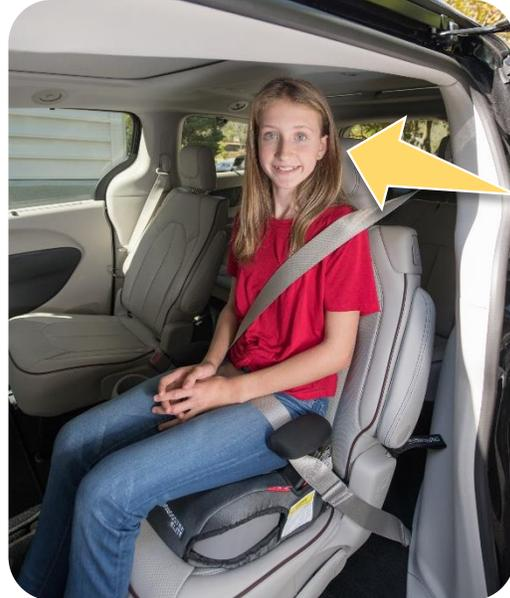
This child is too big for a booster seat. The tops of their ears are above the top of the vehicle head restraint.
