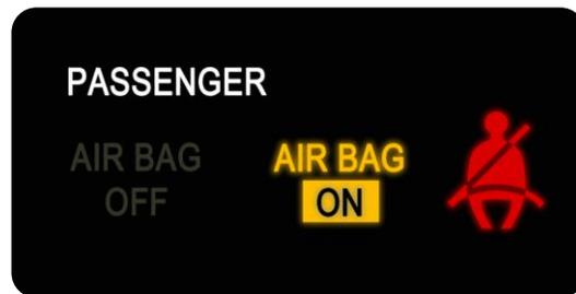
Vehicle dashboard notifications of passenger air bag status, based on sensors
