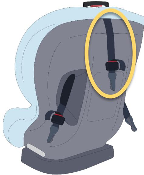
Tether designs vary but all have a standardized hook on a length of webbing that is tightened and loosened using an adjuster.
