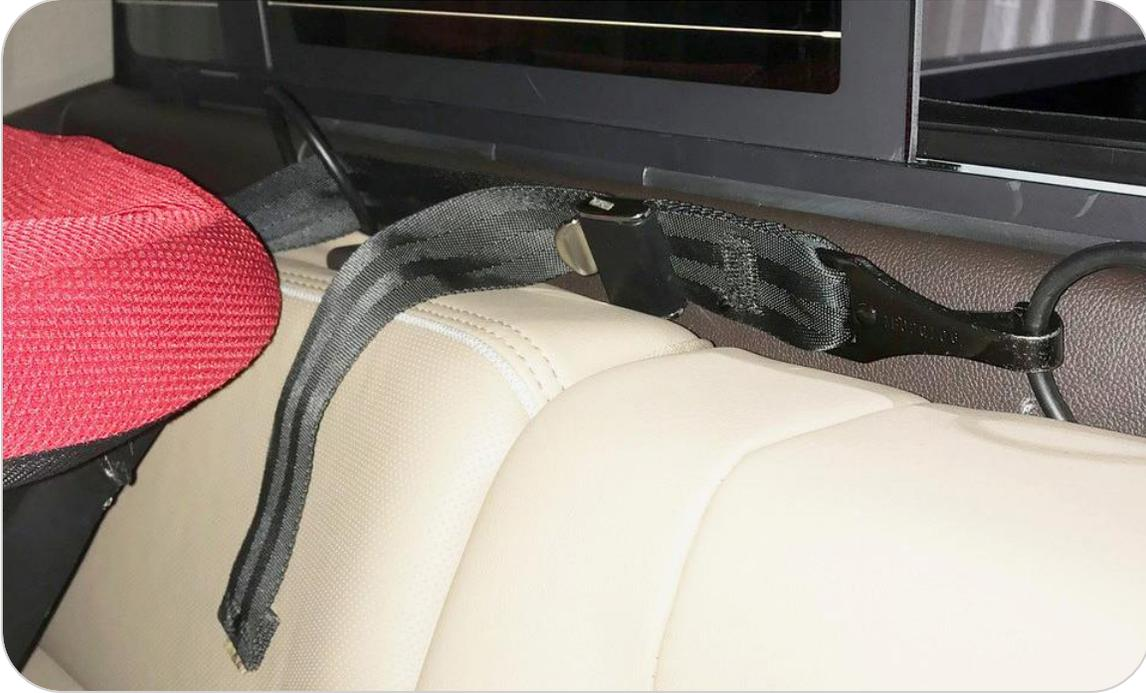
Example of indirect routing in a pickup truck
