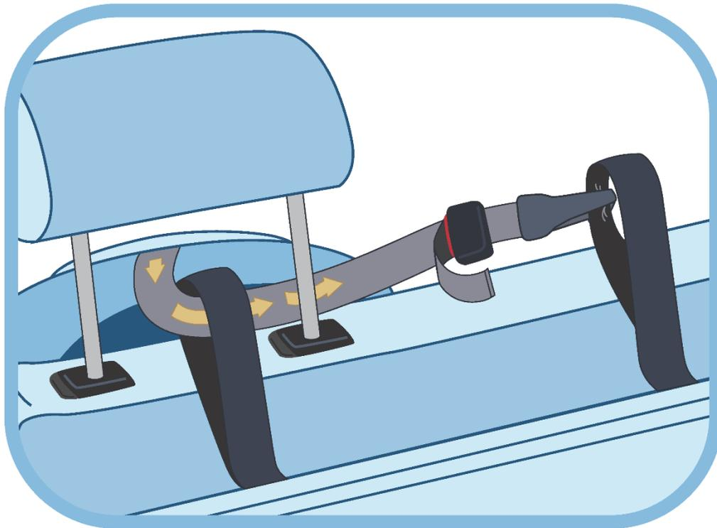
This drawing, from a viewpoint looking through the back window, shows tethering using an indirect routing tether system with a dual-loop design. The tether routes through a loop behind the car seat (the router) and hooks to a loop behind the adjacent vehicle seat (the tether anchor). After attachment, the tether should be tightened.
