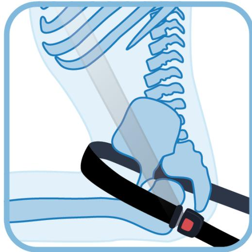
Correct placement of lap belt on child correctly seated on vehicle seat
